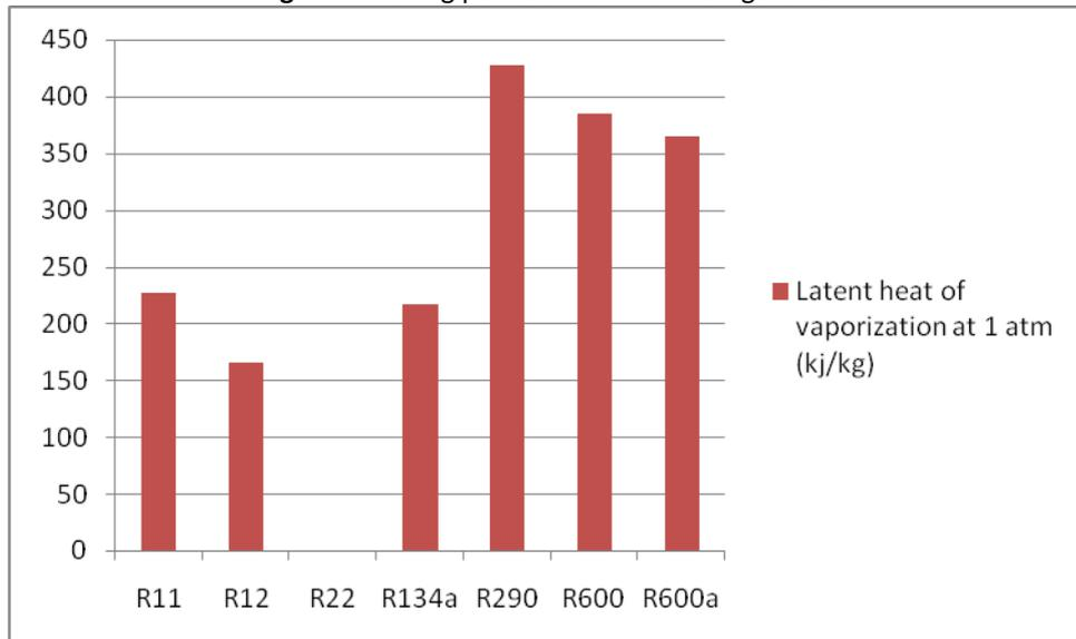
Figure 2: Latent heat of vaporization of common refrigerants
